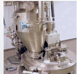
Vapor filter on the headplate
