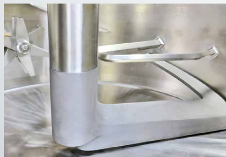
Ceramic plasma coating for wear protection
