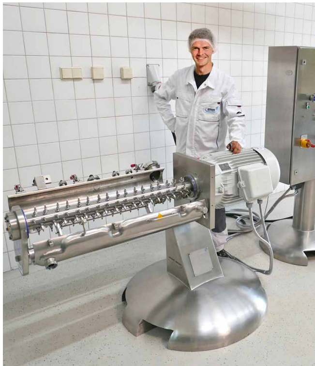
At the end of the amixon® granulator, a balance between grain build-up and grain destruction has been created. If operated ideally, the apparatus produces a soundly compacted granulate within narrow grain size boundaries.
