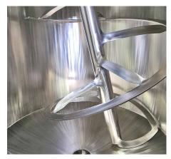
The base has the shape of a dome segment. The mixing goods are mixed without dead space. If desired, they can even be completely discharged using ComDisc®.
