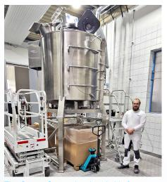
The Gyraton® test mixer is suitable for batches of up to 3 m<sup>3</sup>. Gas-tight, hygienic, universally applicable.
