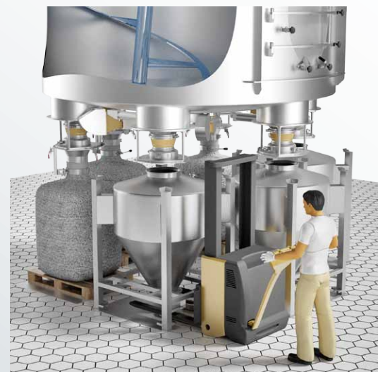
Dispensing can be accelerated if several discharge devices are installed.
